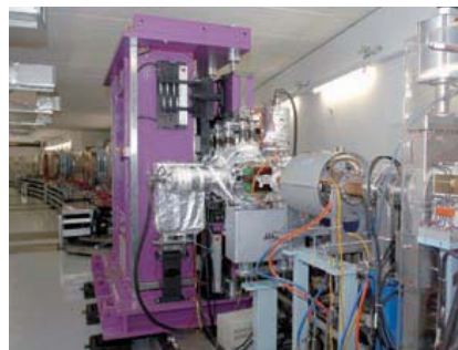
• The in-vacuum undulator designed by SSRF
